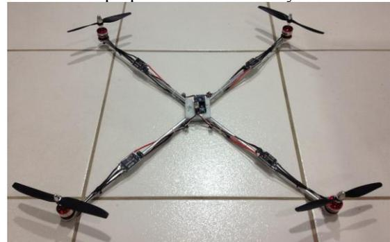
Fig. 2 Modeled quadcopter
